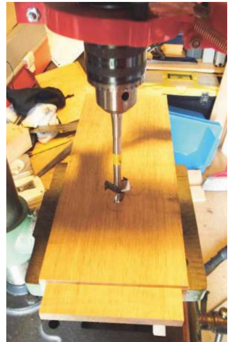
▲ Pic.9 Forstner bit mounted in a bench drill
